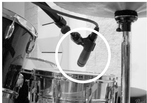
Image 9: Example of snare drum mic placement
